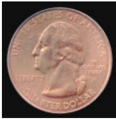
Figure 2. Obverse clad-layer missing.
