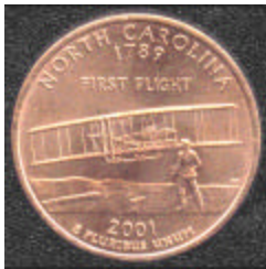
Figure 3. Reverse clad-layer missing.
